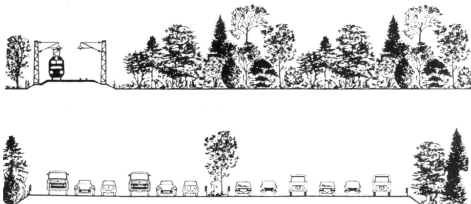
Figure II.2.7.3.i.: Land occupation of modern railways and motorways, calculated for equal transportation performance
