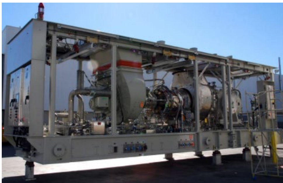
33. Figure: The compressor and the gas turbine are built into a common cabin, container [3]
