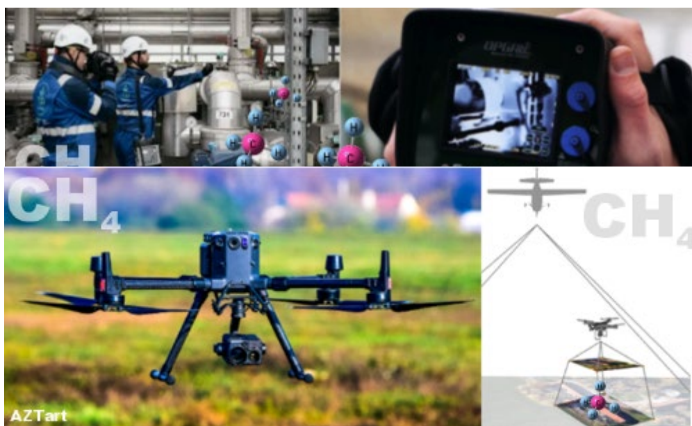
10. Figure: By installing LDAR cameras on drones and collecting remote data, leak detection can be organized on a regular basis, even in the entire extent of natural gas pipelines [4]
