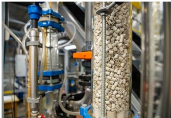
49. Figure: BC cracker catalysts, pilot plant
