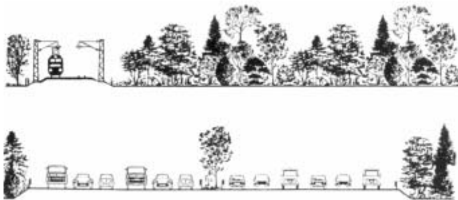
Figure 2.3.f.: Land occupation of modern railways and motorways, calculated for equal transportation performance
